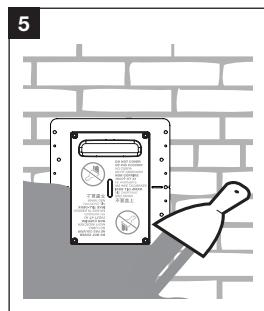
Make sure that the thickness of the plaster is flush with the inlet (about 1 cm) all around the inlet (figure 6).
