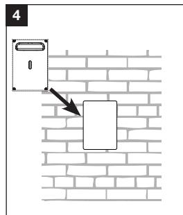
Insert the back of the inlet into the wall and screw the frame of the inlet directly to the brick (figure 5).
