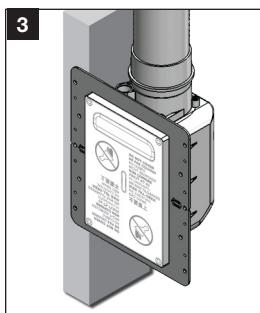
Install the pipe into the fitting (figure 3). Glue the pipe into the fitting, making sure it sits all the way to the ridge of the pipe fitting (see page 11).
