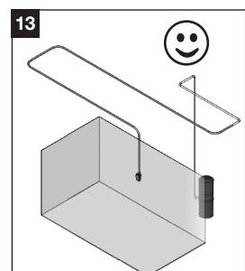
It is important to design the pipe runs so the hose is stored on one level (figure 13). Avoid storing hose on two different levels (figure 14).
