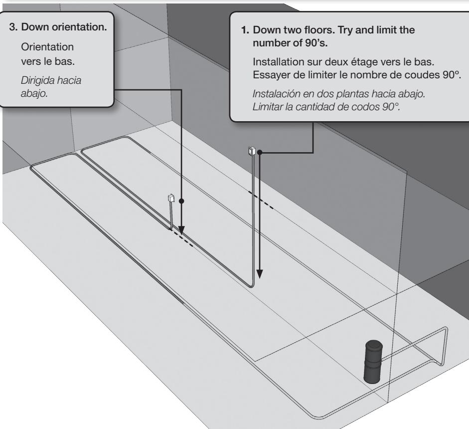
In order to ensure enough pipe to store the hose, the pipe runs will sometimes need to be diverted in order to lengthen piping, and then head back to the power unit.
