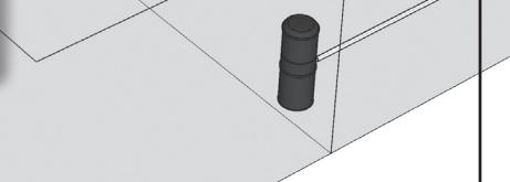
Do not join pipe run until you have enough pipe length to hold the hose, plus an extra length of 20% or 10' (3.05 m) minimum. For example, if using a 60' (18.3 m) hose, install at least 72' (21.9 m) of pipe before connecting to another pipe run.
